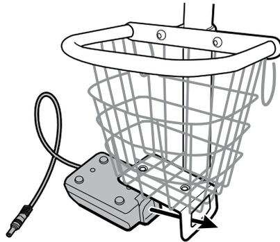
2. Holding the power supply unit snugly to the frame, attach the power supply to the bracket using the 2 Phillips screws.
